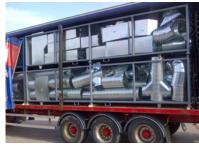
Specially designed and fabricated, 6m long baskets are being used in Dundee for the delivery of ductwork to the New Southern General Hospital in Glasgow.
